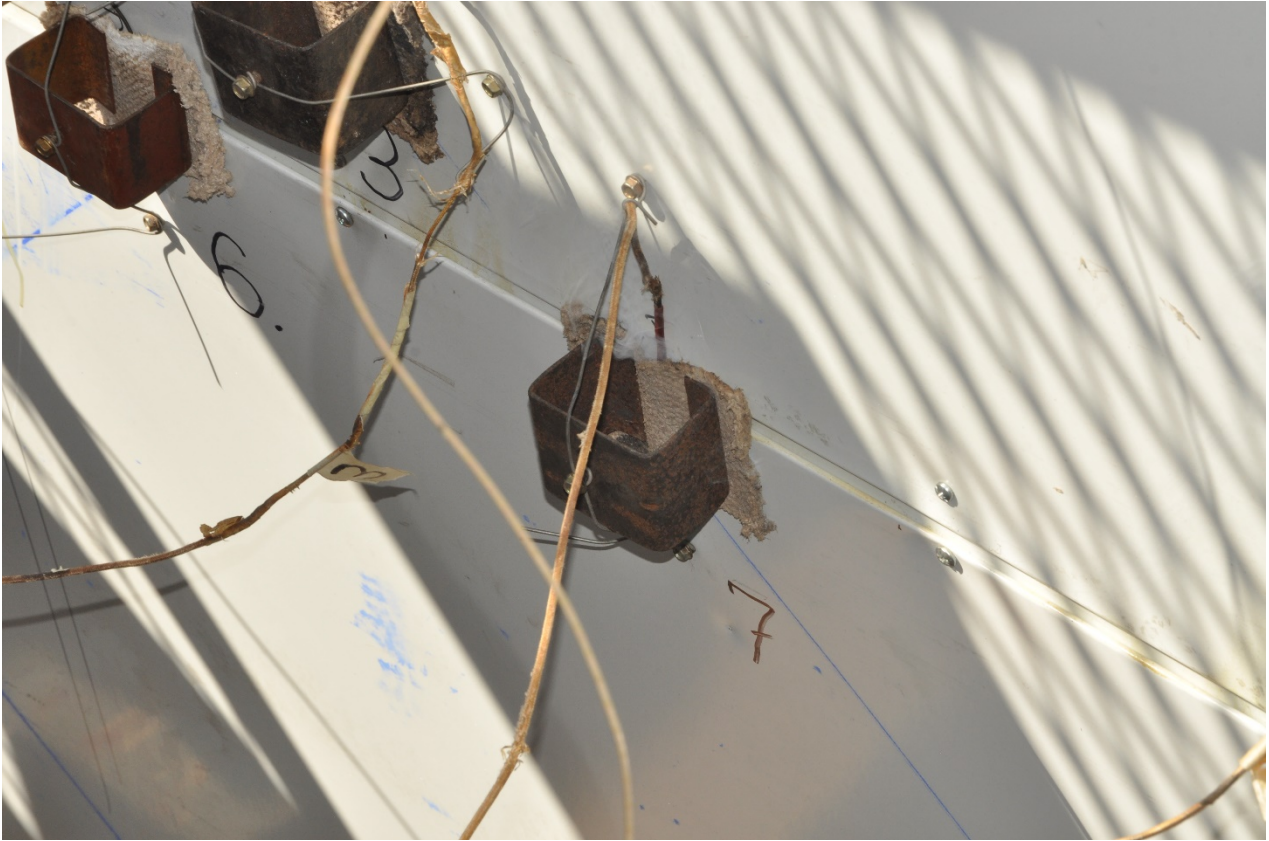
Figure 3.10: Smoke release from TC 7 (bottom joint)
